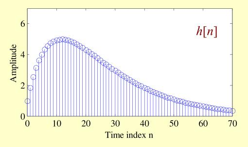
As can be seen from the above plot, the impulse response coefficient h[n] decays rapidly to zero value as n increases
