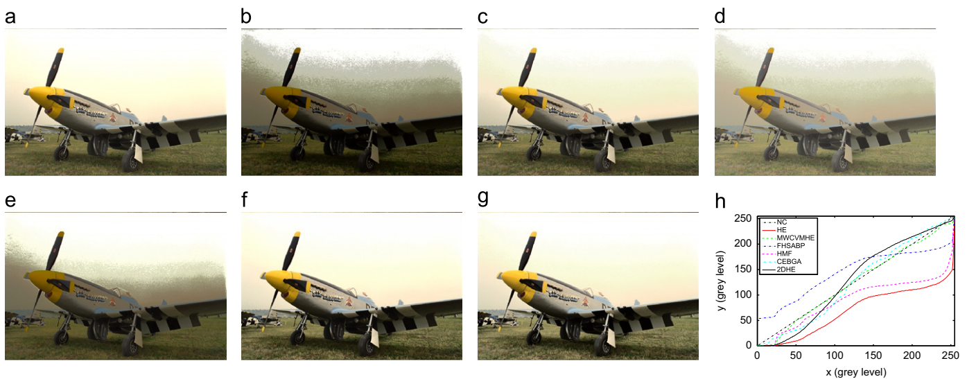
Fig. 8. Contrast enhancement results for image Cessna . (a) Original image. Enhanced images obtained using: (b) HE; (c) MWCVMHE; (d) FHSABP; (e) HMF; (f) CEBGA; and (g) 2DHE. Input to output grey-level mapping functions of enhanced grey-scale images are shown in (h) where “NC” refers to no-change mapping. (For interpretation of the references to color in this figure caption, the reader is referred to the web version of this article.)
