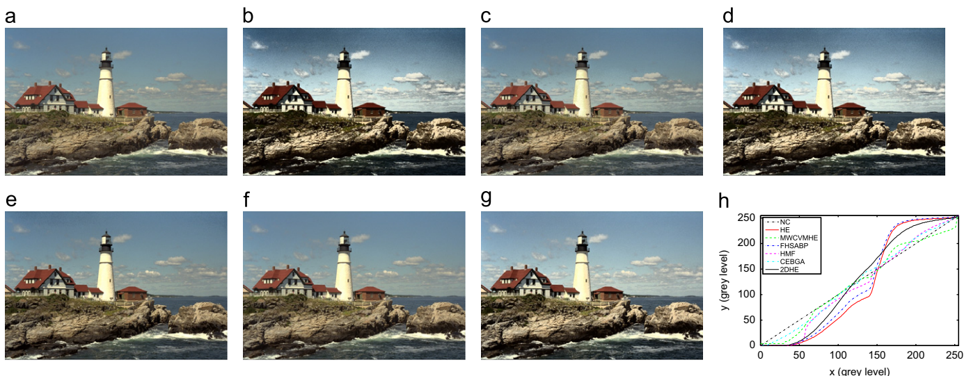
Fig. 9. Contrast enhancement results for image Lighthouse . (a) Original image. Enhanced images obtained using: (b) HE; (c) MWCVMHE; (d) FHSABP; (e) HMF; (f) CEBGA; and (g) 2DHE. Input to output grey-level mapping functions of enhanced grey-scale images are shown in (h) where “NC” refers to no-change mapping. (For interpretation of the references to color in this figure caption, the reader is referred to the web version of this article.)
