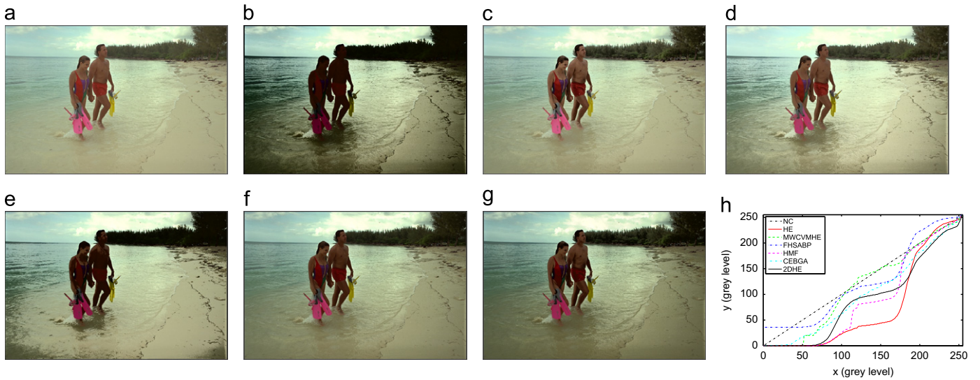
Fig. 10. Contrast enhancement results for image Beach . (a) Original image. Enhanced images obtained using: (b) HE; (c) MWCVMHE; (d) FHSABP; (e) HMF; (f) CEBGA; and (g) 2DHE. Input to output grey-level mapping functions of enhanced grey-scale images are shown in (h) where “NC” refers to no-change mapping. (For interpretation of the references to color in this figure caption, the reader is referred to the web version of this article.)
