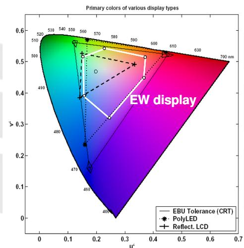
Figure 7 – Color gamut of the three-layer electrowetting architecture, compared to reflective LCD, OLED and EBU.
