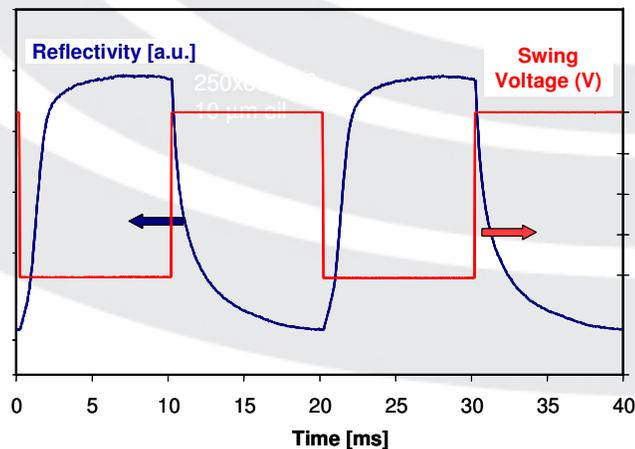
Figure 8 – Response transient of electrowetting display pixels.
