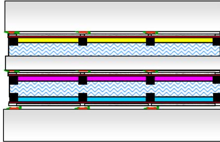
Figure 6 – triple-layer architecture with CMY dyes (not to scale).
