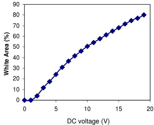
Figure 9 – Electro-optic response of 160x160  $\mu\text{m}^2$  pixels.
