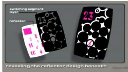
Figure 13 - Display model, showing the switching segment layer and the reflector separately, illustrating the large design freedom.
