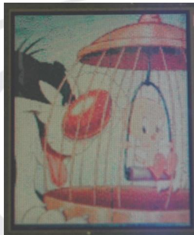
Figure 14 – 1,8" full color active matrix electrowetting display.
