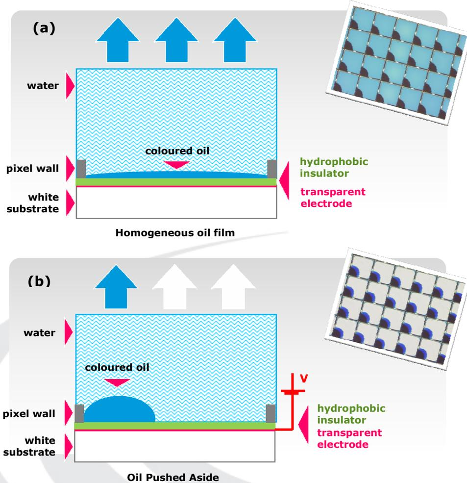
Figure 3 – Electrowetting display principle.
