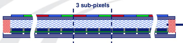
Figure 5 – Single layer architecture with black dye and RGB color filter (not to scale).
