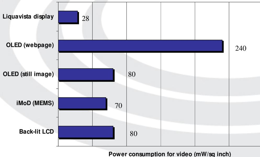
Figure 11 – Comparison of power consumption for a variety of video displays.
