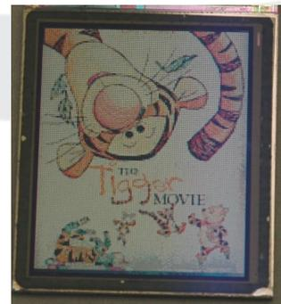
Figure 10 – 1.8" Active matrix display showing 6-bit grey-scale (256k colors) obtained by pulse width modulation.
