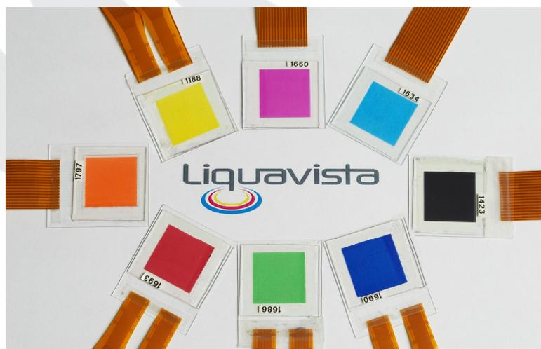
Figure 4 – Color palette for electrowetting displays.
