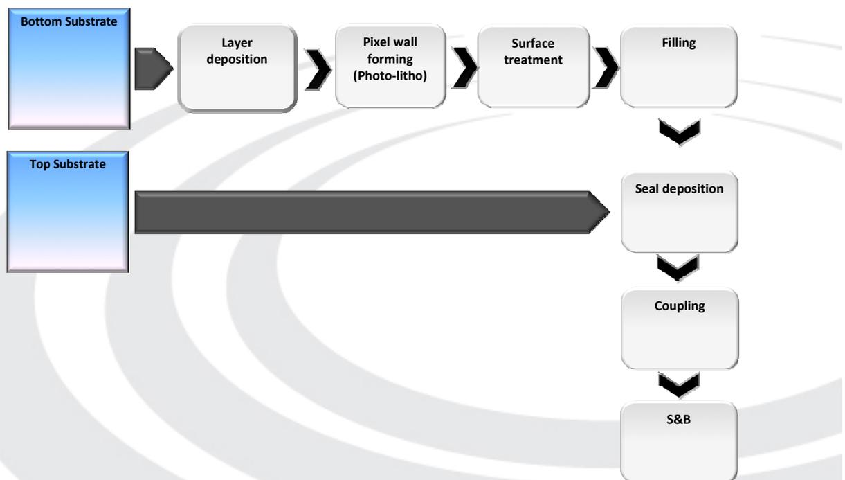
Figure 15 – Process flow for manufacturing electrowetting displays.
