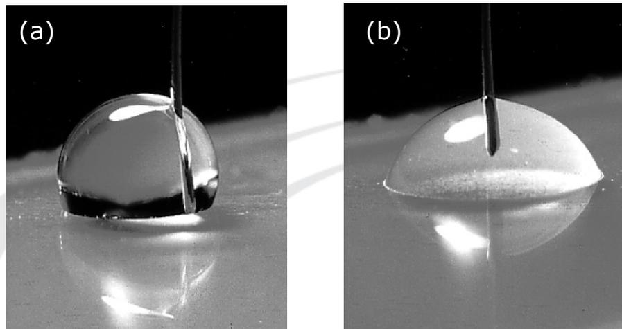
Figure 1 – water droplets on hydrophobic surface (a) without and (b) with voltage applied.
