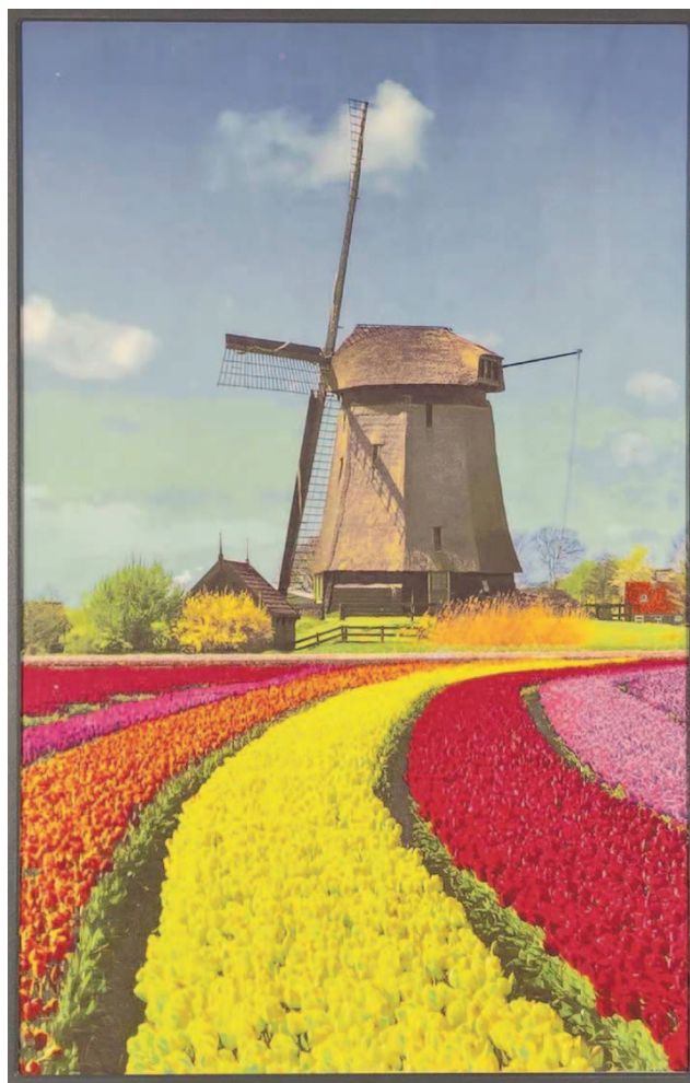
Figure 3. Photograph of an image rendered on a TFT-driven ACEP display module using dithering with 32 device primary colors
