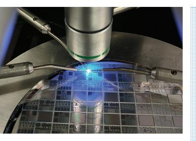
**CLOSE UP:** Lumiode employees examine a wafer containing microLEDs and thin-film transistors.
