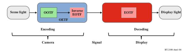
The HLG system was designed with the model shown below, where the OOTF is considered to be in the display.
