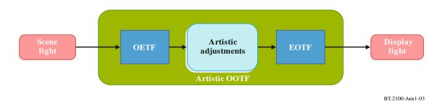
The PQ system was designed with the model shown below, where the OOTF is considered to be in the camera (or imposed in the production process).
