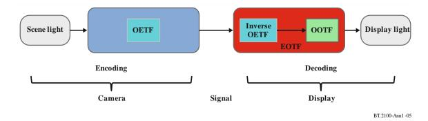
Only two of three non-linearities, the OETF, the EOTF, and the OOTF, are independent. In functional notation (where subscripts indicate the colour component):
