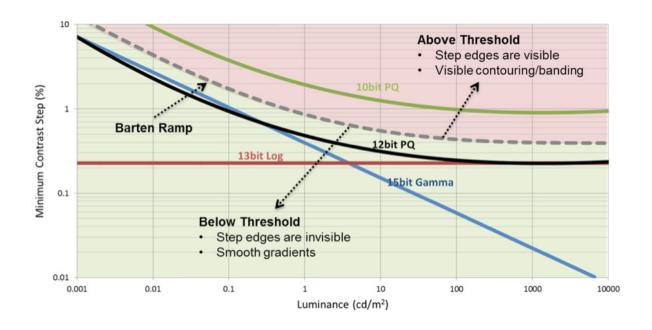
This is a good match for existing cinema infrastructures, and many video-on-demand systems are capable of supplying 12-bit signals as well. Even though 12 bits are required for completely imperceptible steps with noise-free images, the 10-bit PQ curve is only slightly above the Barten Ramp line. In practical systems that include low levels of noise, including sensor noise from cameras, 10-bit PQ has proven itself to be a good match.
