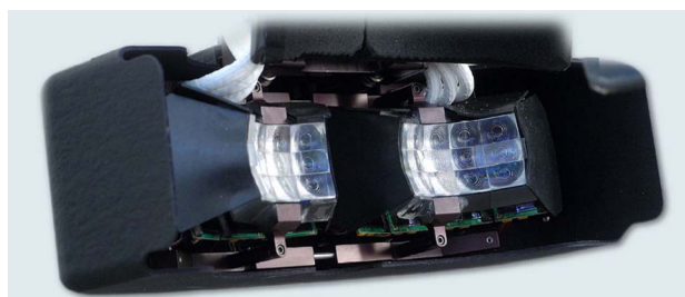
Fig. 5. The Sensics piSight HMD showing tiled microdisplays. Image courtesy of Sensics Inc.
