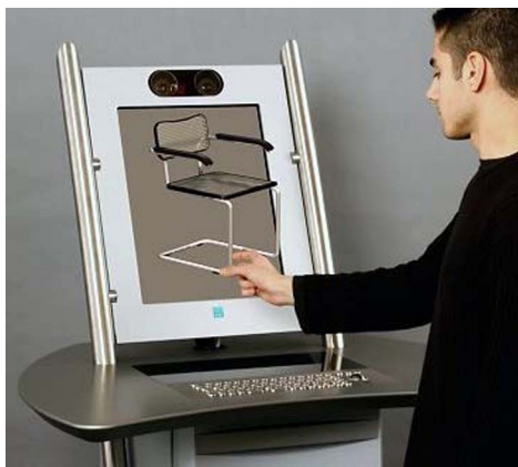
Fig. 10. Free2C interactive kiosk. User handling a multimedia application on the computer without using keyboard or mouse made possible with contact-free interaction technology and autostereoscopic displays.
