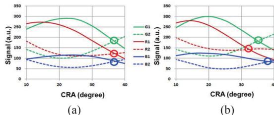
Figure 5. AF crop point measured at horizontal edge of image with (a) in-pixel DTI separation (b) PN junction separation where solid line and dotted line represent left and right signal respectively.
