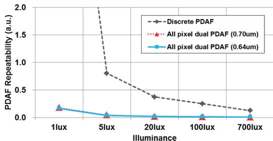
Figure 4. PDAF repeatability of conventional discrete PDAF and dual PD CIS. Lower repeatability represents better AF performance.
