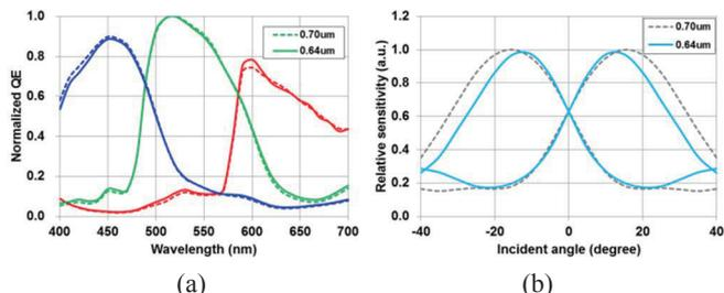
Figure 6. Comparison between  $0.70\mu\text{m}$  and  $0.64\mu\text{m}$  dual PDCIS with (a) normalized QE and (b) AF angular response.
