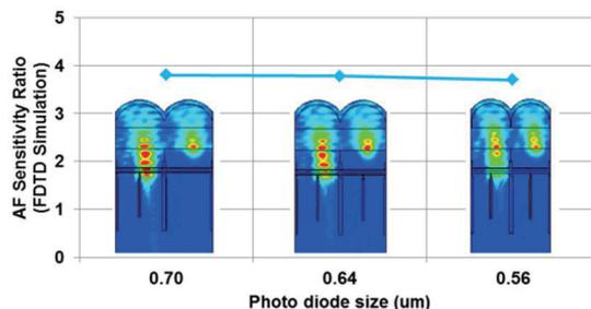
Figure 8. FDTD simulation result of AF sensitivity ratio as the pixel scales down.
