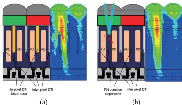
Figure 2. Schematic diagram and optical simulation of PD to PD separation by (a) in-pixel DTI and (b) PN junction.
