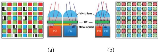
Figure 1. Schematic diagram of (a) conventional discrete PDAF CIS and (b) all pixel dual PD CIS.
