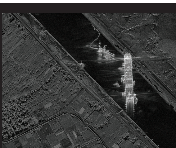
In March 2021, the container ship Ever Given ran aground in the Suez Canal for six days. This satellite image of the ship, captured by synthetic-aperture radar, shows the kind of resolution that is possible with this technology.
