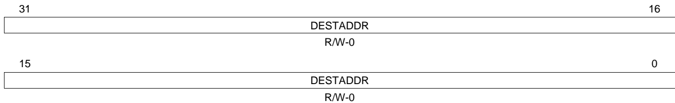
Figure 5-11. IDMA Channel 1 Destination Address Register (IDMA1_DEST)
