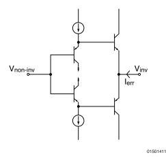
FIGURE 6. Typical CFB Amplifier Input Stage
