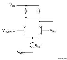
FIGURE 5. Typical VFB Input Stage
