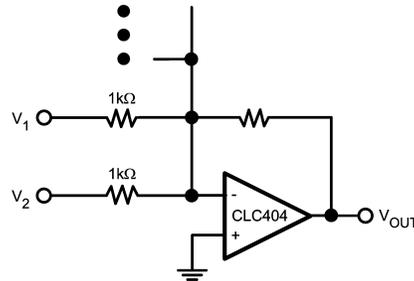
$$V_{OUT} = -(V_1 + V_2 \dots)$$
