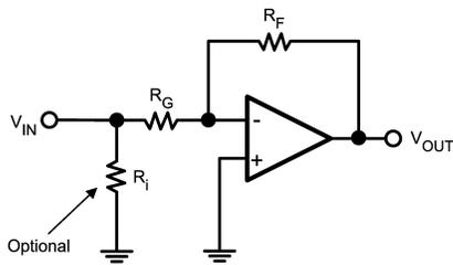
$$V_{OUT} = \frac{R_F}{R_G} V_{IN}$$
