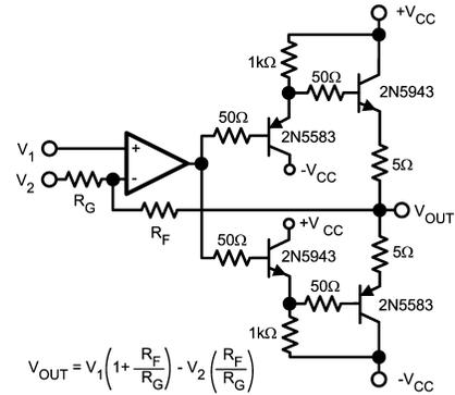
$$V_{OUT} = V_1 \left( 1 + \frac{R_F}{R_G} \right) - V_2 \left( \frac{R_F}{R_G} \right)$$
