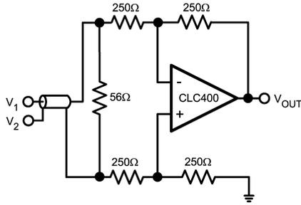
$$V_{OUT} = (V_2 - V_1)$$
