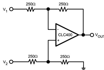
$$V_{OUT} = (V_2 - V_1)$$
