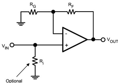
$$V_{OUT} = \left(1 + \frac{R_F}{R_G}\right) V_{IN}$$
