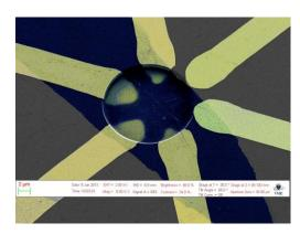
The PhD project is aimed at the development of a graphene-based nanomechanical sensor platform for extremely sensitive protein detection. Single layer graphene sheets will be deposited on a nanofabricated substrate in string or drum configuration (see figure). The predefined electrical contacts will be used to investigate the mechanical properties of the devices in vacuum and in liquid.
