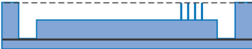
Figure 2c. Pumping Chamber/Filter Etch. Etch a rectangular pumping chamber with Acoustic Terminator at fill end.
