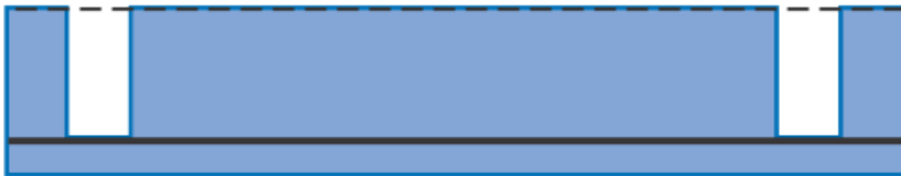
Figure 2b. Descender/Fill etch. Etch blind holes. This Descender will connect the pumping chamber to the nozzle. The Fill connects to fluid reservoir.
