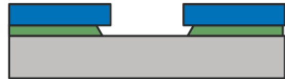
4. Develop resist and LOR or PMGI. LOR or PMGI develops isotropically, creating a bi-layer re-entrant sidewall profile.
