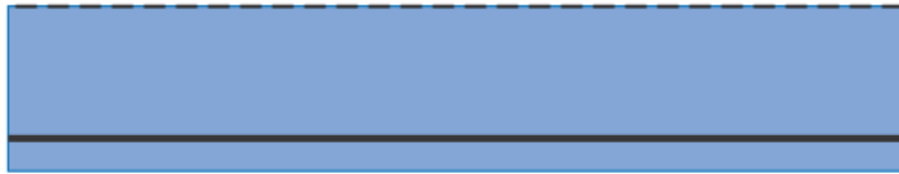
Figure 2a. Starting Wafer. Begin with a Silicon-on-Oxide (SOI) Wafer.
