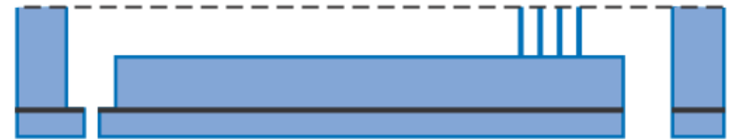
Figure 2d. Nozzle/Fill Through Etch. Etch a through hole to complete nozzle and fill paths.
