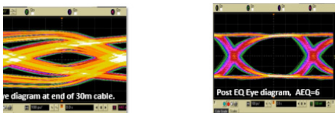
Figure 8. Contrast Between Closed (left) and Open (right) Eye Diagrams
